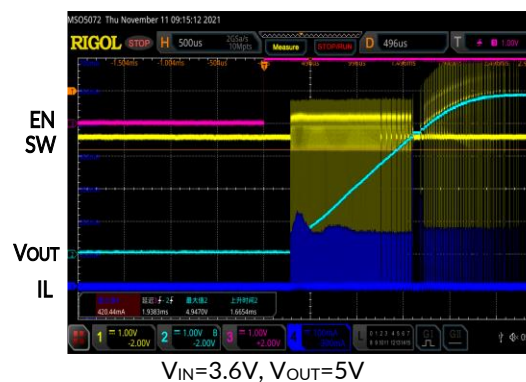
Figure 10. Start - Up after Enable
