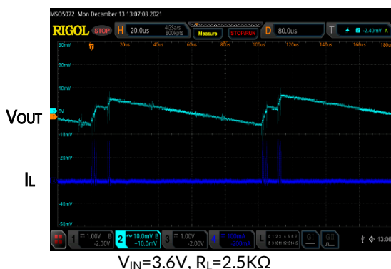
Figure 11. Output Voltage in Power-Save Mode
