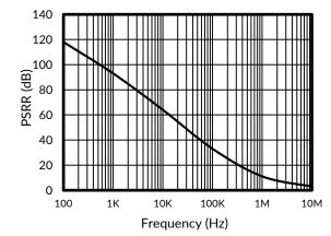
Figure 5. Power-Supply Rejection Ratio vs Frequency
