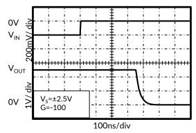
Figure 13. Positive Overvoltage Recovery
