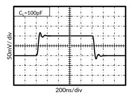
Figure 11. Small-Signal Step Response
