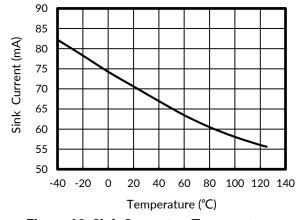
Figure 10. Sink Current vs Temperature
