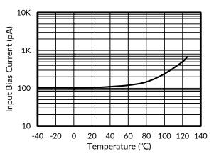
Figure 4. Input Bias Current vs Temperature
