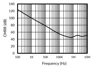
Figure 6. Common-Mode Rejection Ratio vs Frequency
