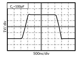
Figure 12. Large-Signal Step Response
