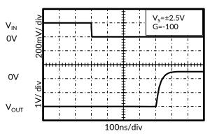
Figure 14. Negative Overvoltage Recovery
