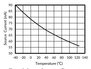
**Figure 9. Source Current vs Temperature**
