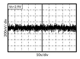
Figure 18. 0.01Hz to 1Hz Noise
