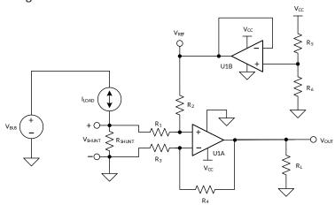
Figure 19. Bidirectional Current-Sensing Schematic
