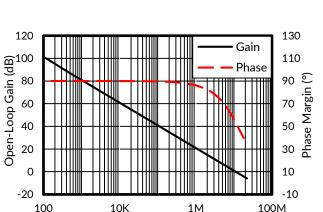
Figure 3. Open-Loop Gain and Phase vs Frequency
