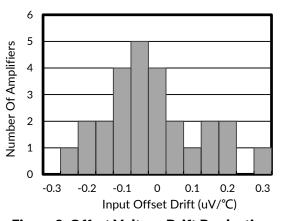
Figure 2. Offset Voltage Drift Production Distribution
