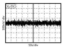
Figure 17. 0.01Hz to 1Hz Noise
