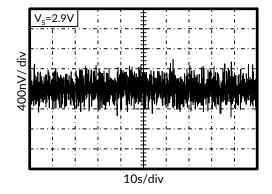
Figure 16. 0.01Hz to 10Hz Noise
