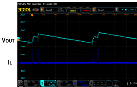
Figure 11. Output Voltage in Power-Save Mode
