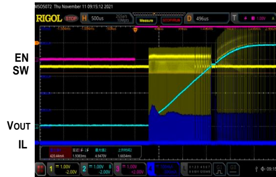
Figure 10. Start-Up after Enable
