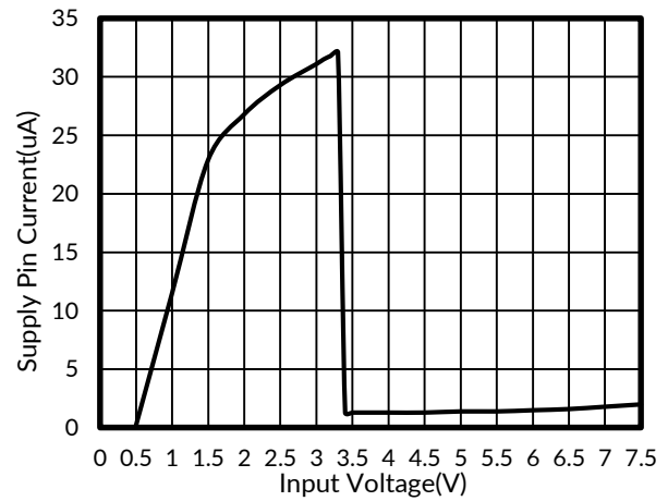
Figure 7. Supply pin Current vs Input Voltage
