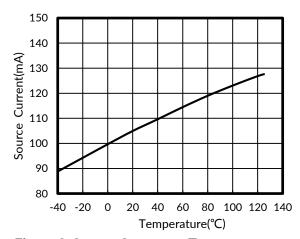
Figure 8. Source Current vs Temperature
