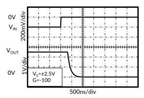
Figure 12. Positive Overvoltage Recovery
