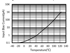
Figure 9. Input Bias Current vs Temperature
