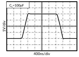
Figure 11. Large-Signal Step Response
