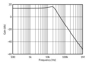
Figure 19. Low-pass filter transfer function
