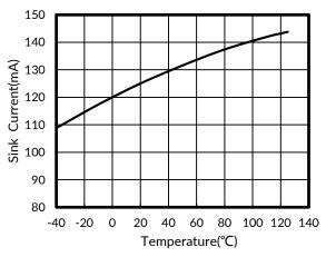
**Figure 7. Sink Current vs Temperature**
