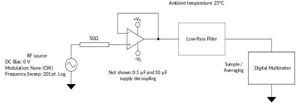
Figure 17. EMIRR IN+ Test Configuration Schematic
