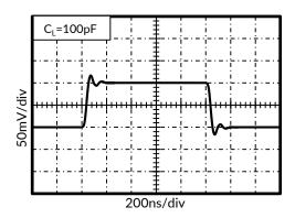
Figure 10. Small-Signal Step Response
