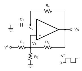
**Figure 1. Square Wave Generator Schematic**
