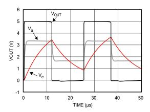
Figure 3. Square Wave Oscillator Output Waveform
