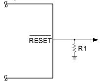
Figure 1. RESET Valid to Ground Circuit
