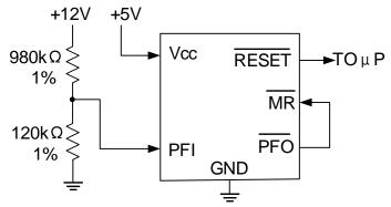
Figure 2. Monitoring Both 5V and 12V
