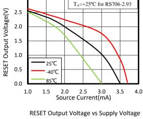
**RESET Output Voltage vs Source Current**
