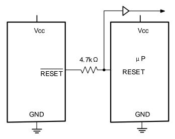
Figure 3. Buffered RESET to other system components
